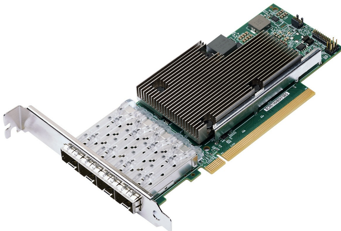
Figure 2. ThinkSystem Broadcom 57454 10/25GbE SFP28 4-port PCIe Ethernet Adapter
