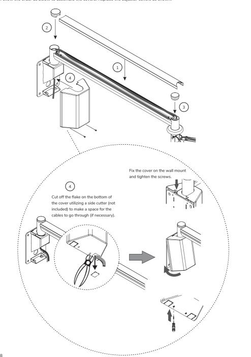
Follow the order as below to assemble the covers. Replace the adjuster covers as shown.
