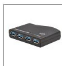
USB 3.2 Gen 1 portable hub adds 4 USB-A ports to your PC, laptop, Chromebook, tablet or other USB-enabled device.
