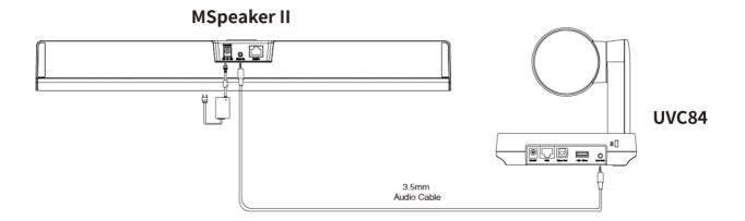
Method 2: Connect to the VCH port of the UVC camera/AVHub:
