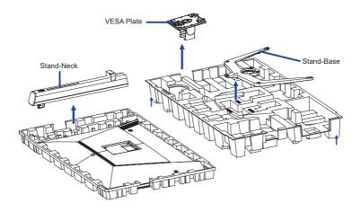
3 Attach the Stand-Neck to the VESA Plate and then tighten the 'thumb screw' with the provided screwdriver to secure them.
