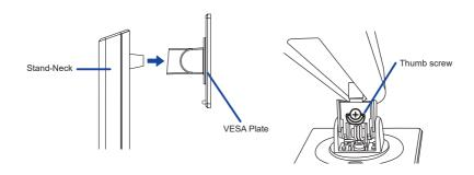
④ Install the Stand-Base to the Stand-Neck and then tighten the 'thumb screw' to secure them.
