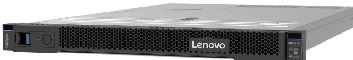
Figure 25. Lockable front security bezel
