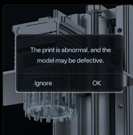
Bottom layer separation inspection, AI detection
